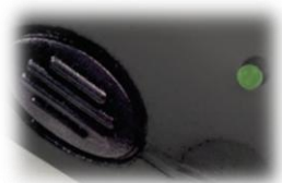
stay-on self timed switch with LED indicator,
