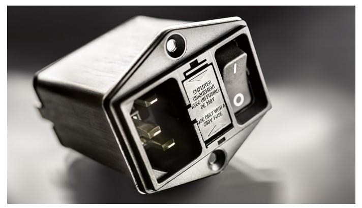
SCHURTER DD14: Combination element consisting of IEC appliance plug, mains switch, fuse holder and double-stage EMC filter
