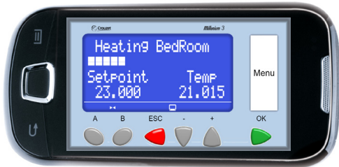
The Millenium 3 screen is transferred to an Android smartphone: example when the logic controller is programmed to monitor the temperature in a room
